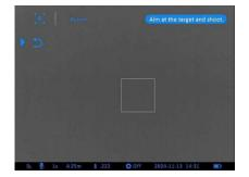
Step 3: Aim at the calibration object or target placed at 25 meters, ensuring the rectangular frame is positioned on the target surface.
