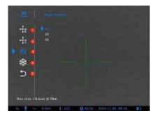
The correction parameter defaults to 0, meaning no adjustment is applied to the reticle position.
