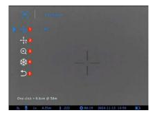
The prompt in the lower left corner indicates the centimeter value represented by each unit of reticle movement at the current distance.
