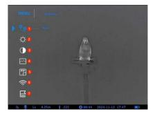
On the observation interface, short press the "Menu Button" to enter the quick menu. The quick menu includes the following options: Reticle Distance Memory, Screen Brightness, Contrast, Scene Mode, PIP, WiFi, Range Settings (Range version)
